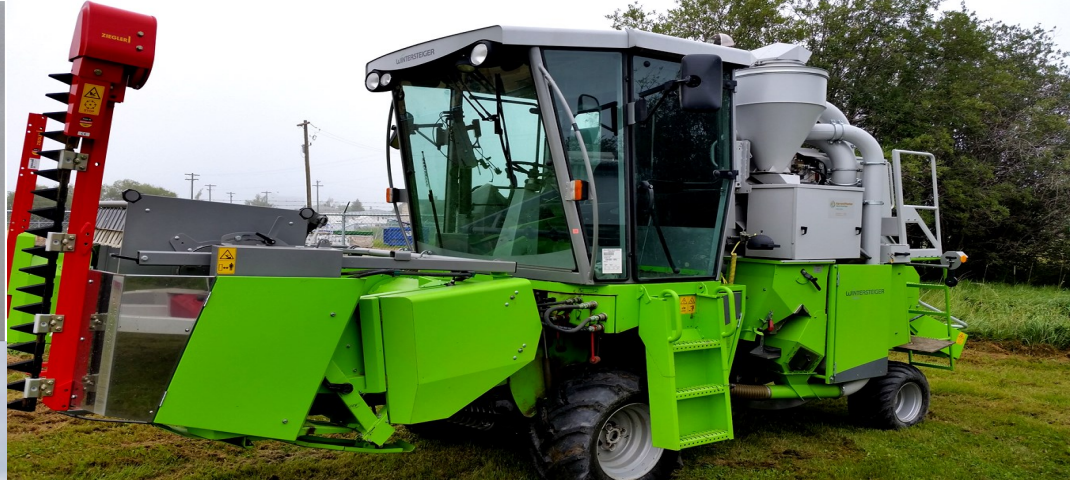
2011 Wintersteiger Plot Combine With straight cut header and vertical cutter bars onboard weigh system pickup header
