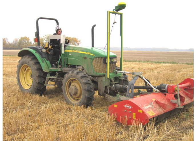
Front Mount PTO Mower with RTK Guidance System
