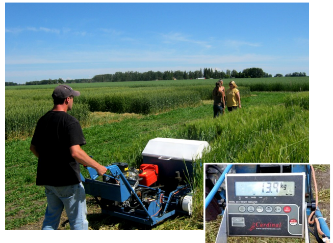
Silage harvester with onboard scale
